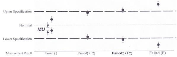
( ) This result is indicated on the measurement report as a blank space in the column labeled "Status" or "Sts". MU = 95% expanded measurement uncertainty.
